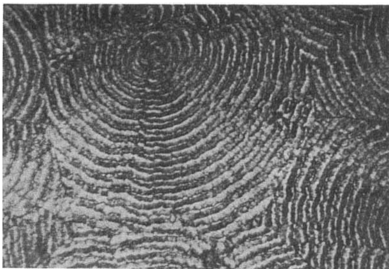
FIGURE 5 Ringed spherulites formed during cold crystallization of 9DDA9-M; magnification \times 320 .
